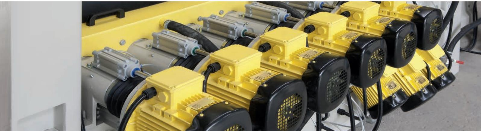
Disruptive electrical discharges found in applications such as electric motors, can cause damage to bearing raceways or disturb signal transmission in encoders. Fast switching frequency converters can account for these discharges, however asymmetrical magnetic flow in the motors and unshielded asymmetrical wires are the two classic causes common in large motors with a low pole pair number, as they have higher magnetic asymmetry than their smaller counterparts.
